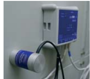
Options include (from top left): ultrasonic microphone, contact ultrasonic sensor and plug-in TEV probe
